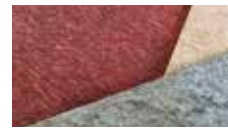
Malai An organic and sustainable biocomposite material made of bacterial cellulose, produced with agricultural waste from the coconut industry in southern India.
