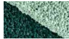
AluFoam An advanced porous metal with the unique benefits of foamed materials and the design flexibility of aluminium
