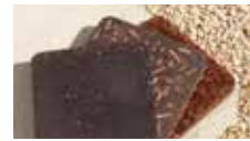
DATEFORM Innovative solid surfaces made from date seeds in the United Arab Emirates
