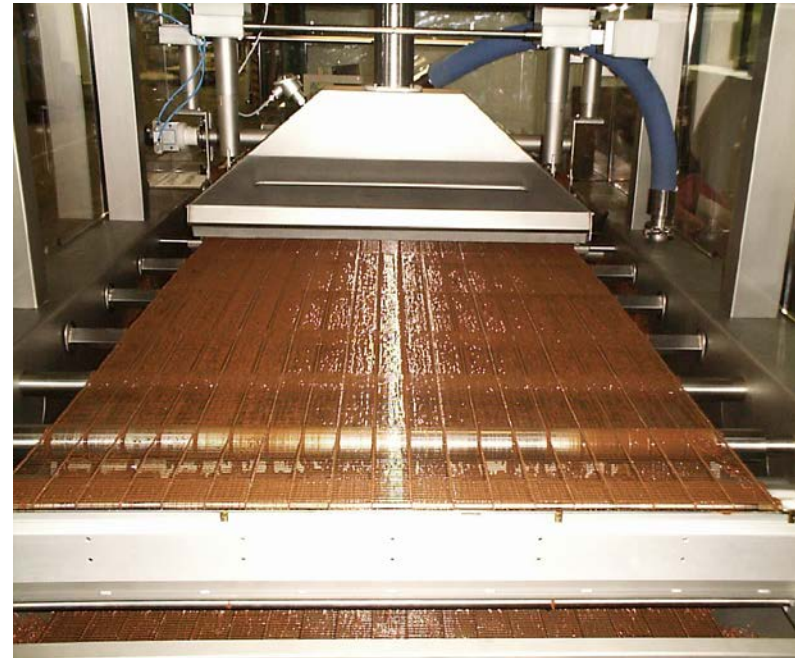
View into Enrober from Discharge
