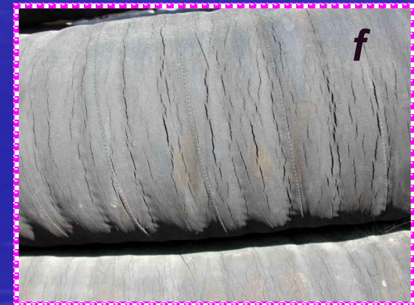
Flexible hoses (NBR) for water drainage from the AST roof: e - fuel oil after 5 y; f - industrial atmosphere after 1 y.
