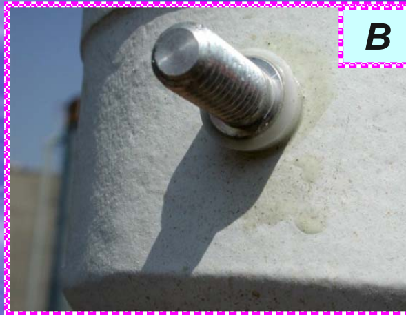
B - an aluminum stub glued to measured coating
