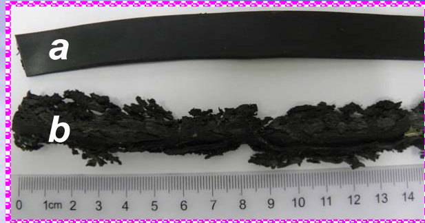
a – original seal (natural rubber); b – after 6 months of service in kerosene.
