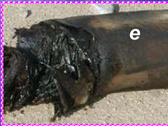
Flexible hoses (NBR) for water drainage from the AST roof: e - fuel oil after 5 y; f - industrial atmosphere after 1 y.
