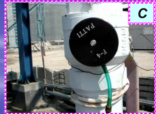
C - measuring of adhesion of coating on the pipe
