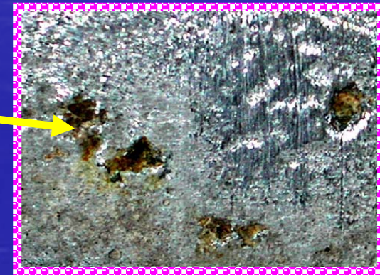
Pontoon made from aluminum alloy Al 5052 after a 3-week hydrotest
