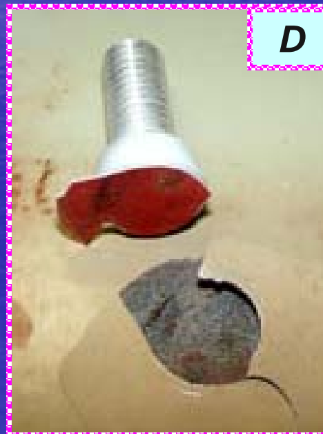
B - an aluminum stub glued to measured coating
