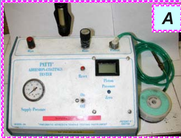
A –PATTI 2 for measuring of adhesion
