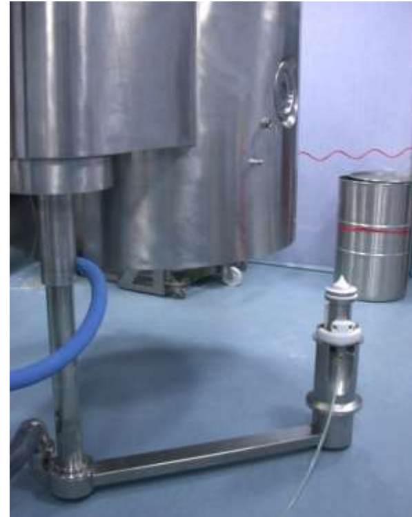
GMP compliant change of spray nozzle – available in-process
