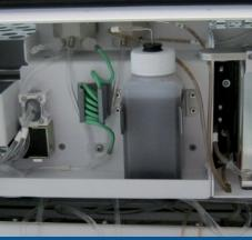
Nitrate module or ISE module for pH, conductivity & redox analysis (options)
