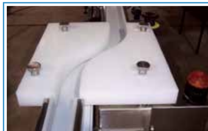
Side-by-side conveyor transfer
