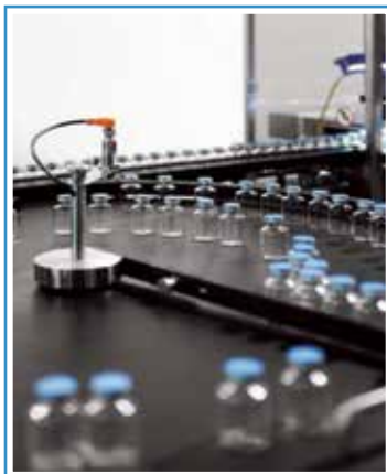
Rotary accumulating and transfer tables
