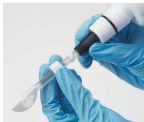
Installation of a general purpose shaft
