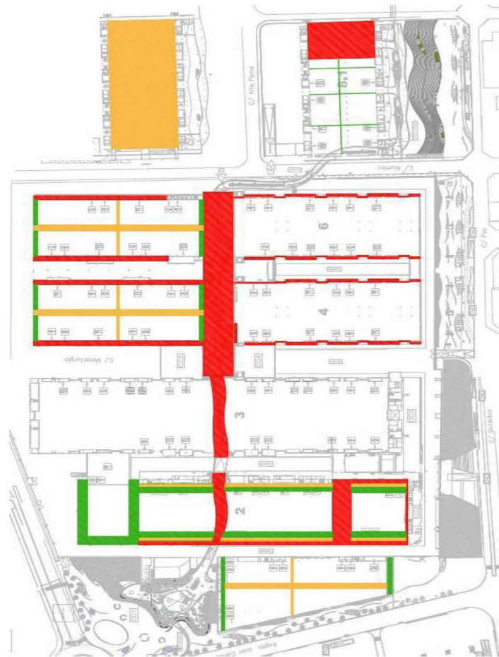
■ Area with special conditions for the placement of the Rigging ■ Area with impossibility to place Rigging ■ Pre-Rigging Area placement of special structure
