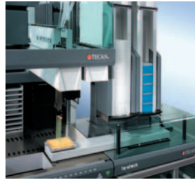
The Te-Stack ensures fast and continuous loading of microplates.
