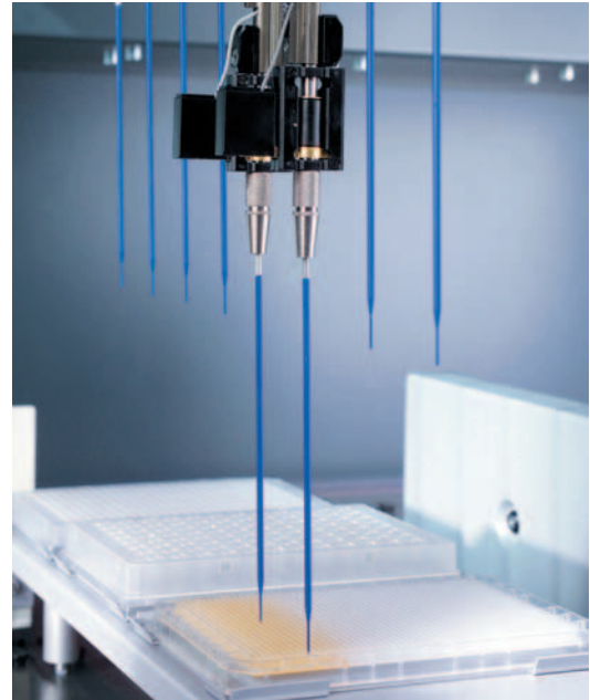
Te-PS (Tecan positioning system) assures reliable and accurate pipetting in 1536-well or protein crystallography plates.
