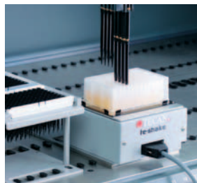
The Te-Shake shakes MTPs, DWPs, Eppendorf as well as PCR tubes.
