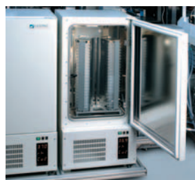
Third party robotic incubators fit beside and underneath the Freedom EVO.
