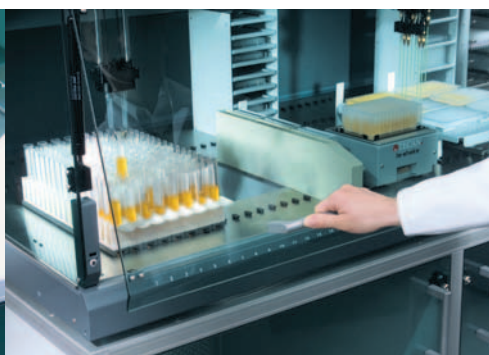
Doorlocks and cover shields prevent unintended access to the worktable during a run.
