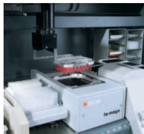
The Te-MagS performs magnetic bead separation.
