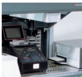
PCR application with integrated thermocycler.
