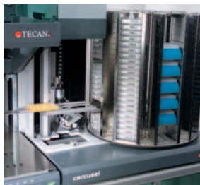
The high speed carousel stores up to 189 microplates.
