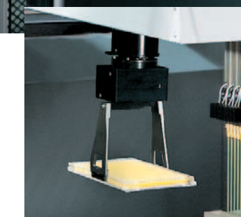
Existing Freedom EVO can be upgraded with a robotic manipulator arm.
