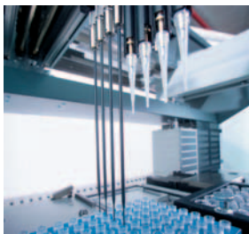
Mixed-tip configuration with disposable and fixed tips.
